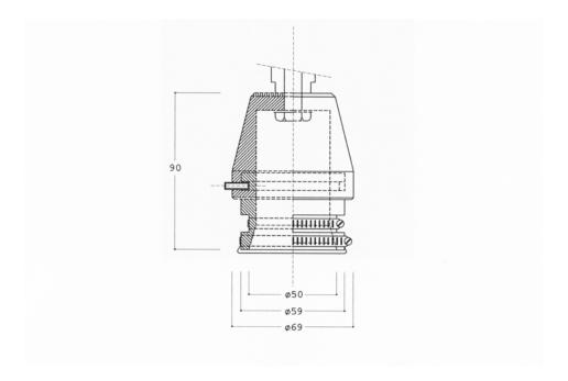
Figure A.5. Fixing device for test of cloth resistance to perforation
