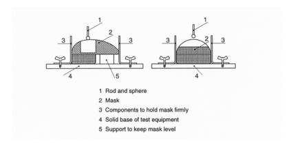
Figure A.2. Method of fixing the mask
