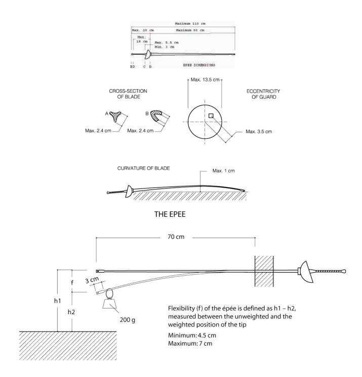
Figure 9. Epee dimensions and flexibility
