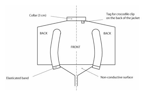
Figure 15. Electric saber conductive jacket
