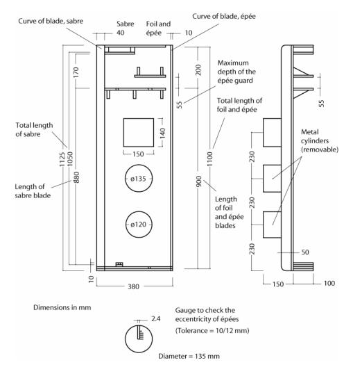
Figure 16. Gauge for checking weapons
