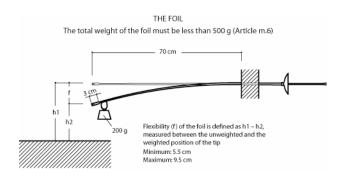
Figure 8. Foil dimensions and flexibility
